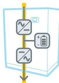
In the event of power supply failure the battery provides power to the inverter, ensuring the required runtime with no interruptions at all.
