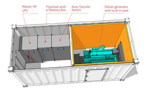
PowerBox is available in different combinations. Below are two examples of installations in 20 and 40-foot containers, with Riello UPS, a flywheel and a diesel generator.
